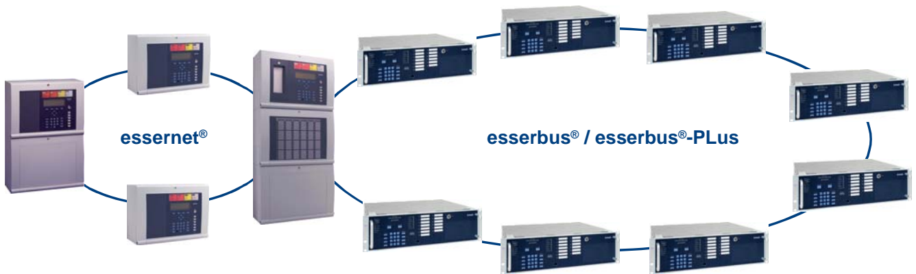
Fig. 50: Operation of the Extinguishing Control Computer in the Fire Alarm System 8000 / IQ8Control
